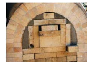
Figure 2a. Refractory lining of a furnace arch (BEE, 2005)
