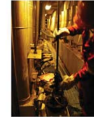
Still have coke formation inside tube after cleaning.
